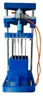
When fixing the Warner bratzler module, insert the blade in the female module, then fix the blade by screwing, and then insert the female module inside the table
